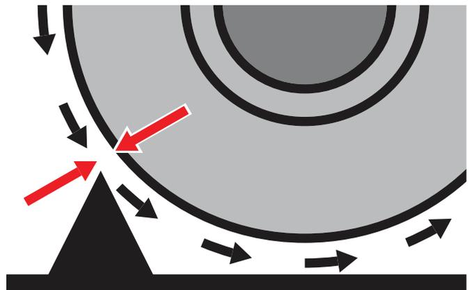
**C Tyre fitting not central on rim.** Check that tyre guide rib is same distance from rim around the entire circumference of rim. 2mm deviation is acceptable. If unacceptable, refit tyre to rim after turning 180°.
